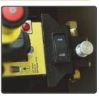
Shown: Control Console Installation of Open/Close Momentary Rocker Switch
