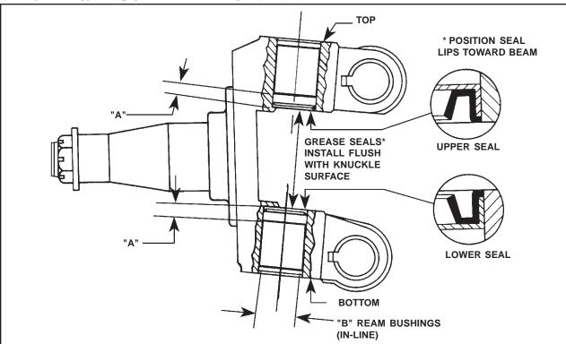
KNUCKLE BUSHING AND KING PIN SEAL INSTALLATION FIG. 2
