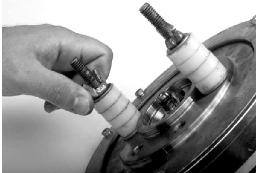
Picture of Compressing the clutch with two 3/8" x 3" bolts
